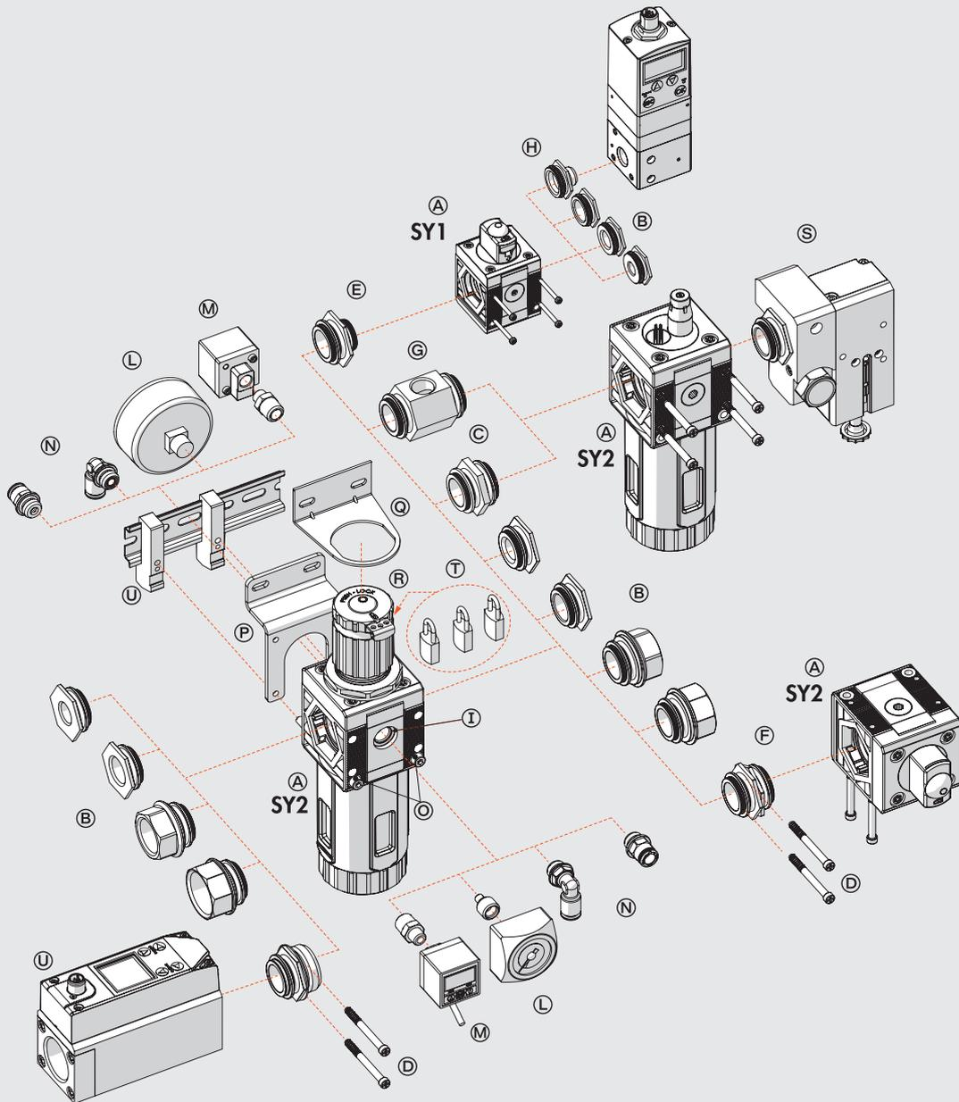
The various elements of Syntesi® A can be connected to the air feed and delivery circuit using pneumatic nickel brass or passivated aluminium ports® and can be fixed together using nipples®.
