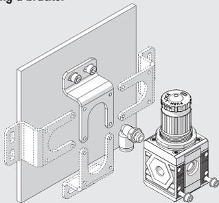
The bracket can be secured in any position, and the fittings can be mounted on the pressure gauge air intake at the back of the unit.
