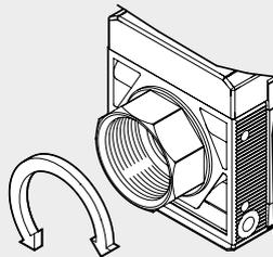
3/4" and 1" bushings in Size 2 rotate freely to facilitate assembly operations.
