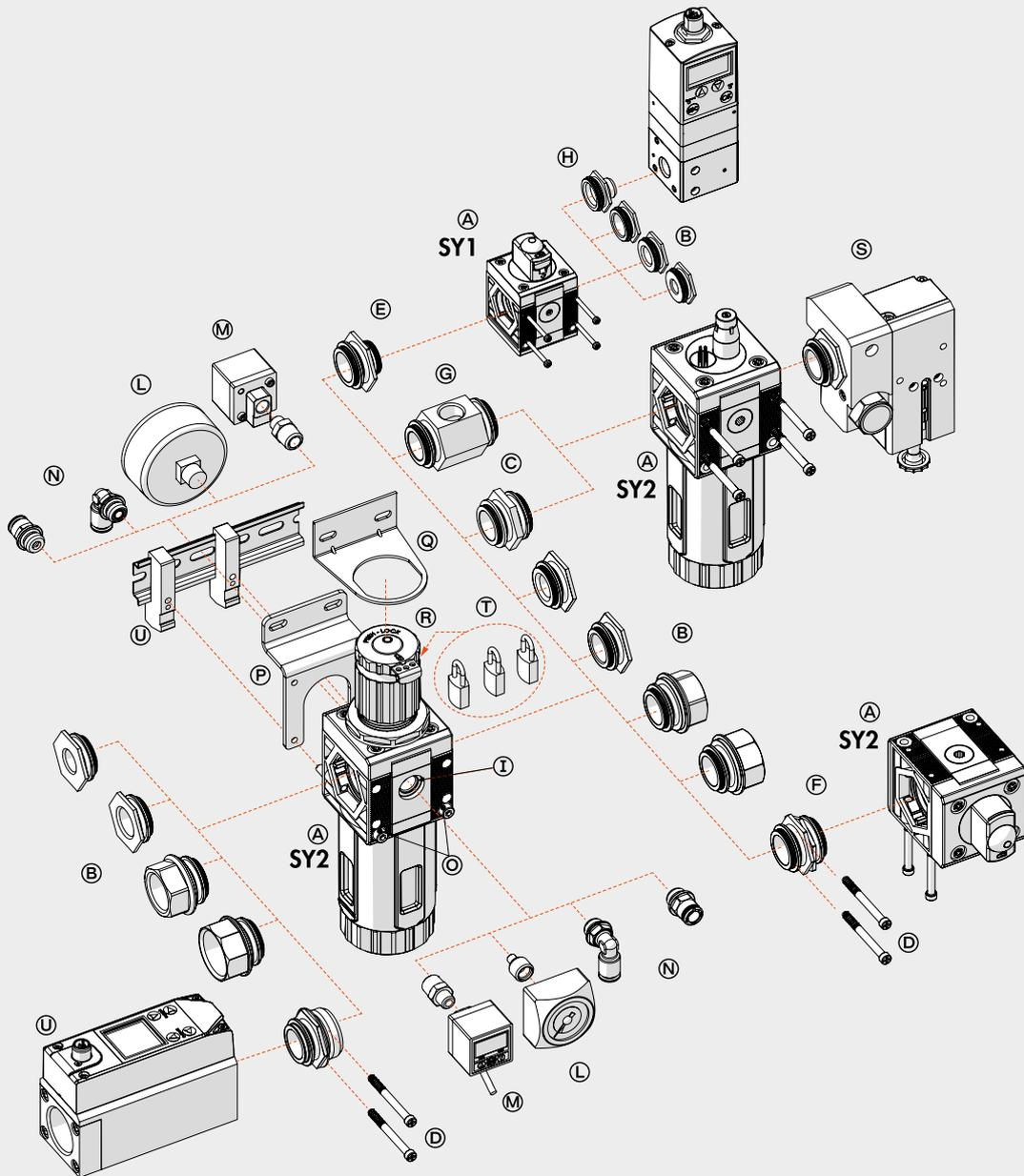
The various elements of Syntesi® ④ can be connected to the air feed and delivery circuit using pneumatic nickel brass or passivated aluminium ports ⑤ and can be fixed together using nipples ⑥.
